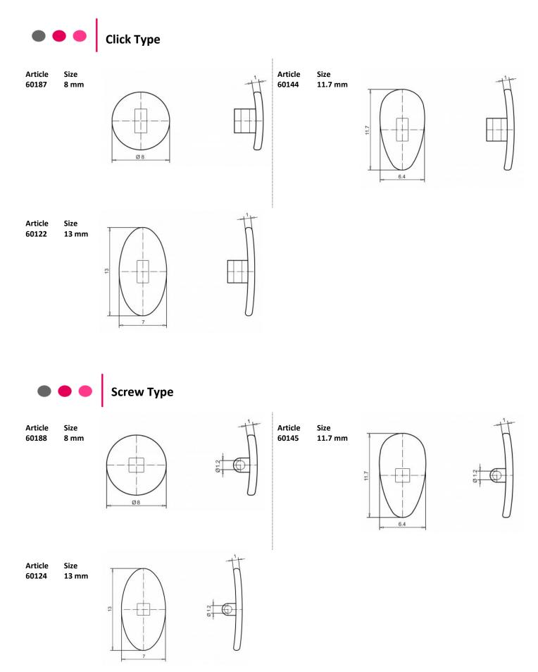
**Body:** Made of titanium grade 1-material, anti-allergic and corrosion-free **Logo/brand:** Logo engraving by laser available on request
